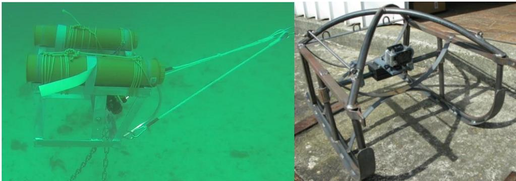
The flying array (left) and the camera sled (right) used for habitat surveys
