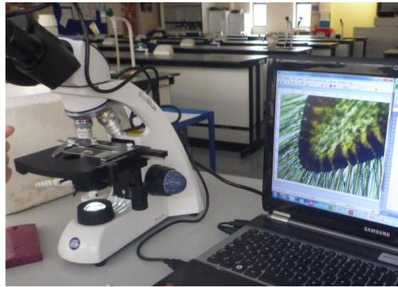
The computer screen shows the image of a lobster pleopod taken using a USB microscope camera for analysis.
